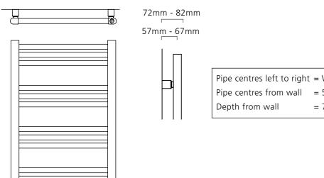
Pipe centres left to right = Width less 44mm = 57mm - 67mm = 72mm - 82mm
